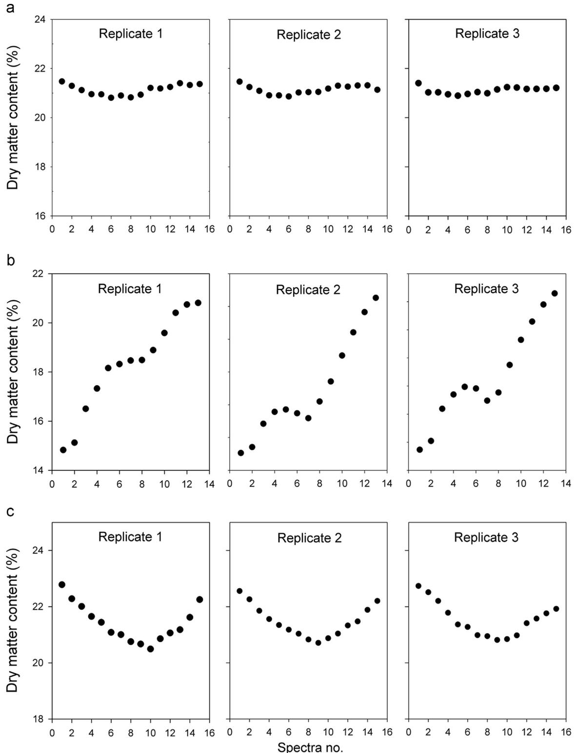
**Fig. 4.** Three different patterns emerged when dry matter content was predicted from the individual spectra recorded from a sample. Note that three replicates are shown side by side. (a) a sample with rather homogenous dry matter content, (b) increasing (or decreasing, if potatoes were turned the other way before measurement) dry matter along the potato length, (c) potatoes with lower dry matter content at the center, and higher dry matter content in the periphery.
