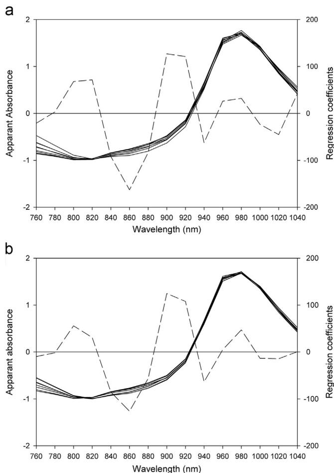
**Fig. 1.** Example spectra (solid lines) and regression coefficients (dotted lines) for the models obtained from the off-line contact (a) and off-line non-contact (b) measurements. Spectra shown are SNV-transformed apparent absorption spectra. The models obtained from contact and non-contact measurements are both made with 5 PLS factors.
