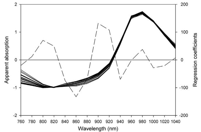
**Fig. 3.** Spectra (solid line) from potatoes moving past the detector. Each spectrum shown contains the averaged spectra from one sample, and is SNV-transformed apparent absorption spectra. Regression coefficients (dotted line) are shown for the prediction model (6 PLS factors) obtained for prediction of dry matter content in potatoes moving along conveyor belt.
