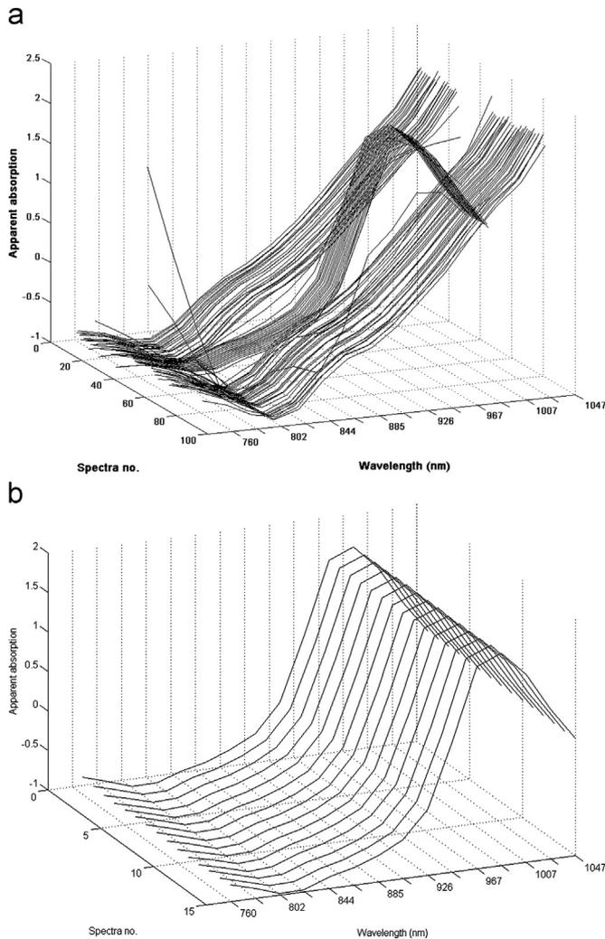
**Fig. 2.** (a) A section of the recording from an on-line measurement of a potato. Spectra with a peak at 950–990 nm represent the potato, the rest of the spectra represent the conveyor belt. All spectra seen are SNV-transformed. The sample shown is from the cultivar Asterix. (b) Spectra remaining after removal of all spectra representing the conveyor belt.
